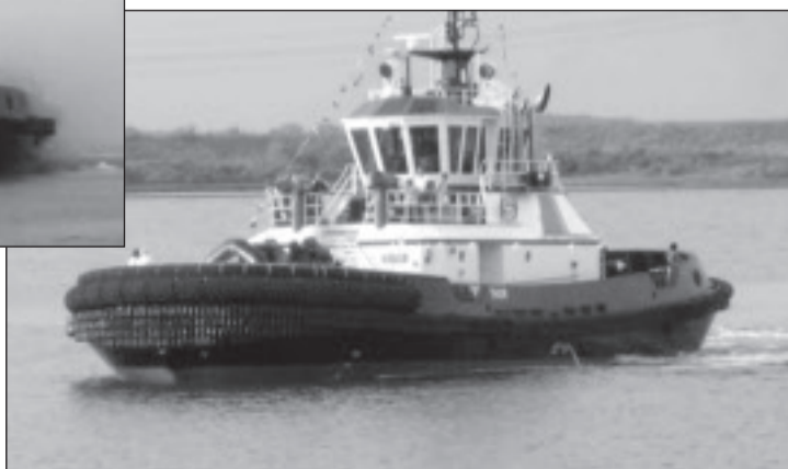
SIU-contracted G&H Towing recently christened the z-drive harbor tug Thor . Seafarers and SIU officials participated in the ceremony at Barbour's Cut in La Porte, Texas. The 6,500 hp tugboat features high-tech navigational and propulsion systems. It also is equipped with a firefighting system that includes a vapor-mist feature designed to extinguish fires on LNG vessels or at LNG terminals. Pictured in the group photo are (from left) SIU Asst. VP Gulf Coast Jim McGee, Mate Travis Parker, DEU Buddy Wheeler, Capt. Doug Caradec, AB Jay Fabian, Relief Capt. Nicoli Payne, Chief Engineer Chris Wootton and SIU VP Gulf Coast Dean Corgey.
