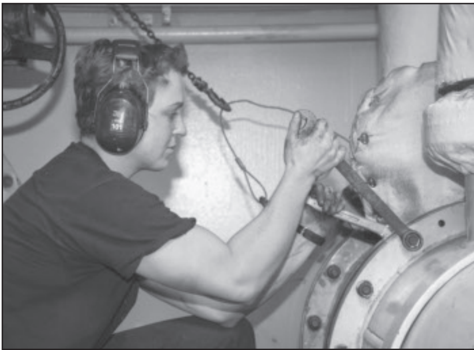
GUDE Monica Coffelt (above) opens a lube oil cooler earlier this year aboard the Lummus . (U.S. Navy photo by Mass Communication Specialist 3rd Class Joshua Fulton) In the photo at right, SIU-crewed prepositioning ships change formation during an exercise off the coast of Saipan. (Photo courtesy of U.S. Navy)
