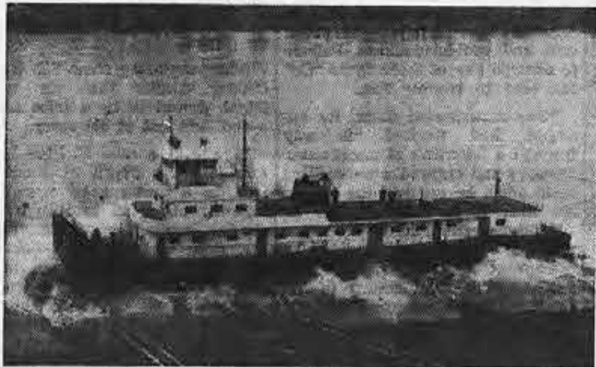
The Clyde Butcher, the newest tug to join the fleet of the SIU Inland Boatmen's Union contracted American Commercial Lines, is shown above during recent launching at Jeffersonville, Indiana. The 5,000 h.p. towboat is 170 feet long, 40 feet in the beam, and draws 11 feet of water. Equipped with twin diesels, the vessel is equipped with the latest instruments for communication, navigation and ship control. She will operate on the Ohio and Mississippi Rivers.
