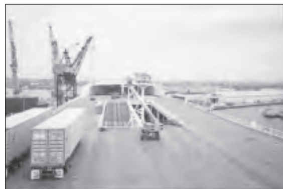
The main deck includes an enclosed bow to provide cover during rough weather.
