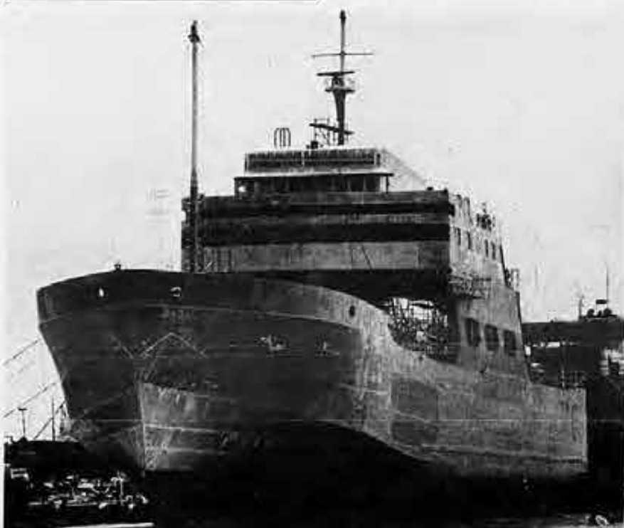
Sacal Borincano, roll on, roll off vessel scheduled to begin operating this month on regular weekly Miami to San Juan, Puerto Rico run for SIU-contracted South Atlantic and Caribbean Line, is world's first large ocean-going commercial vessel with an aluminum hull.
