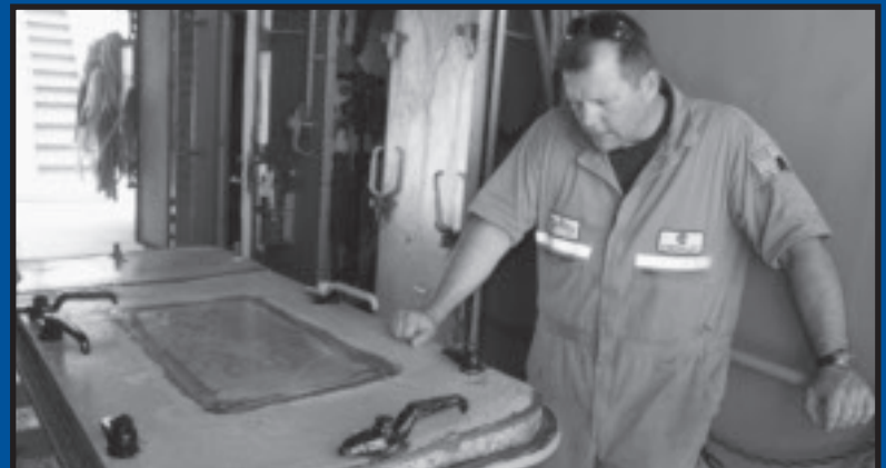
Recertified Bosun Rick James refurbishes a watertight door aboard the Cape Washington .
