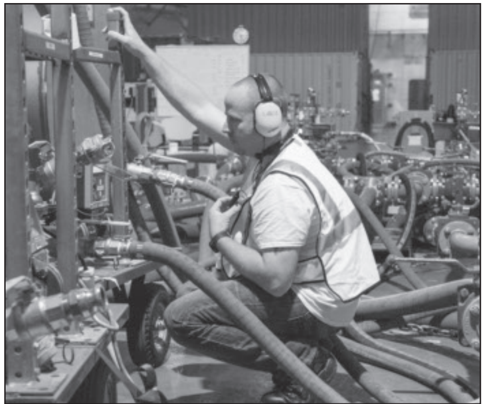
James Lance, a waste handler assigned to the Cape Ray , monitors a hose filling a tank that's part of a field-deployable hydrolysis system installed on the Keystone-operated ship. This mid-June practice operation happened in Rota, Spain.
