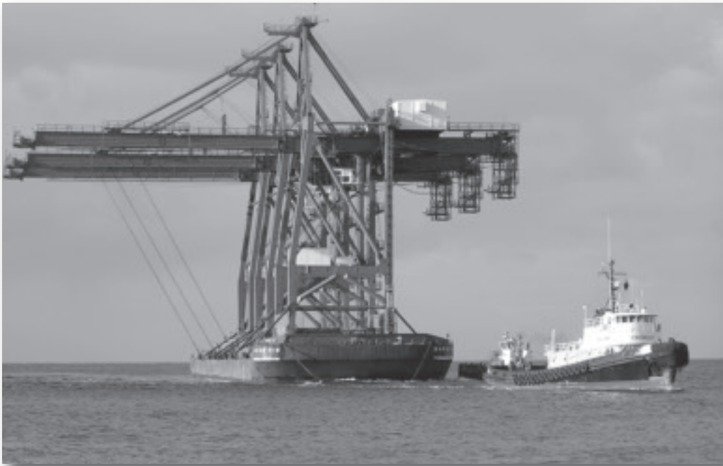
The Seafarers-crewed ocean-going Crowley tug Mars is underway for the port of Apra Guam from Los Angeles. In tow is the 400-foot-long by 100-foot-wide barge 416 which is loaded with three large Hitachi gantry (container) cranes. This voyage marked the second delivery of these types of cranes that Jacksonville, Fla.-based and SIU-contracted Crowley in recent months has made for Bickerton Iron Works, Inc. The first shipment included three cranes which were delivered to the SSA terminal in Manzanillo, Mexico.
