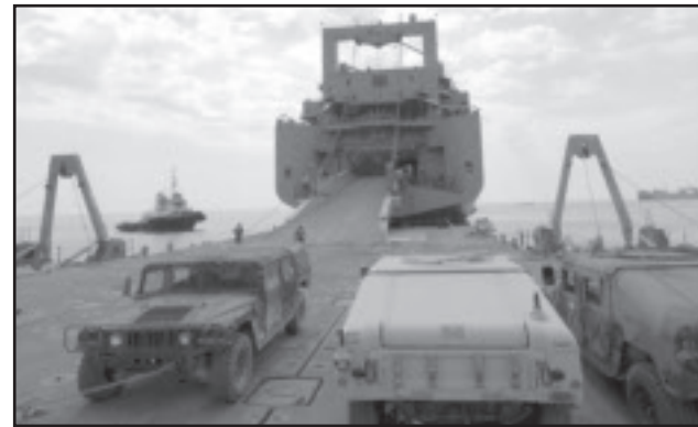
The USNS Soderman 's discharge ramp is used to load equipment onto a Navy lighterage system during an exercise in Guatemala last year.
