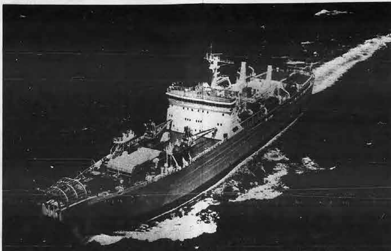
An aerial shot has us looking down onto the deck of the Long Lines where we can see the fore and aft grappling ar J cable laying hatches of the vessel.
