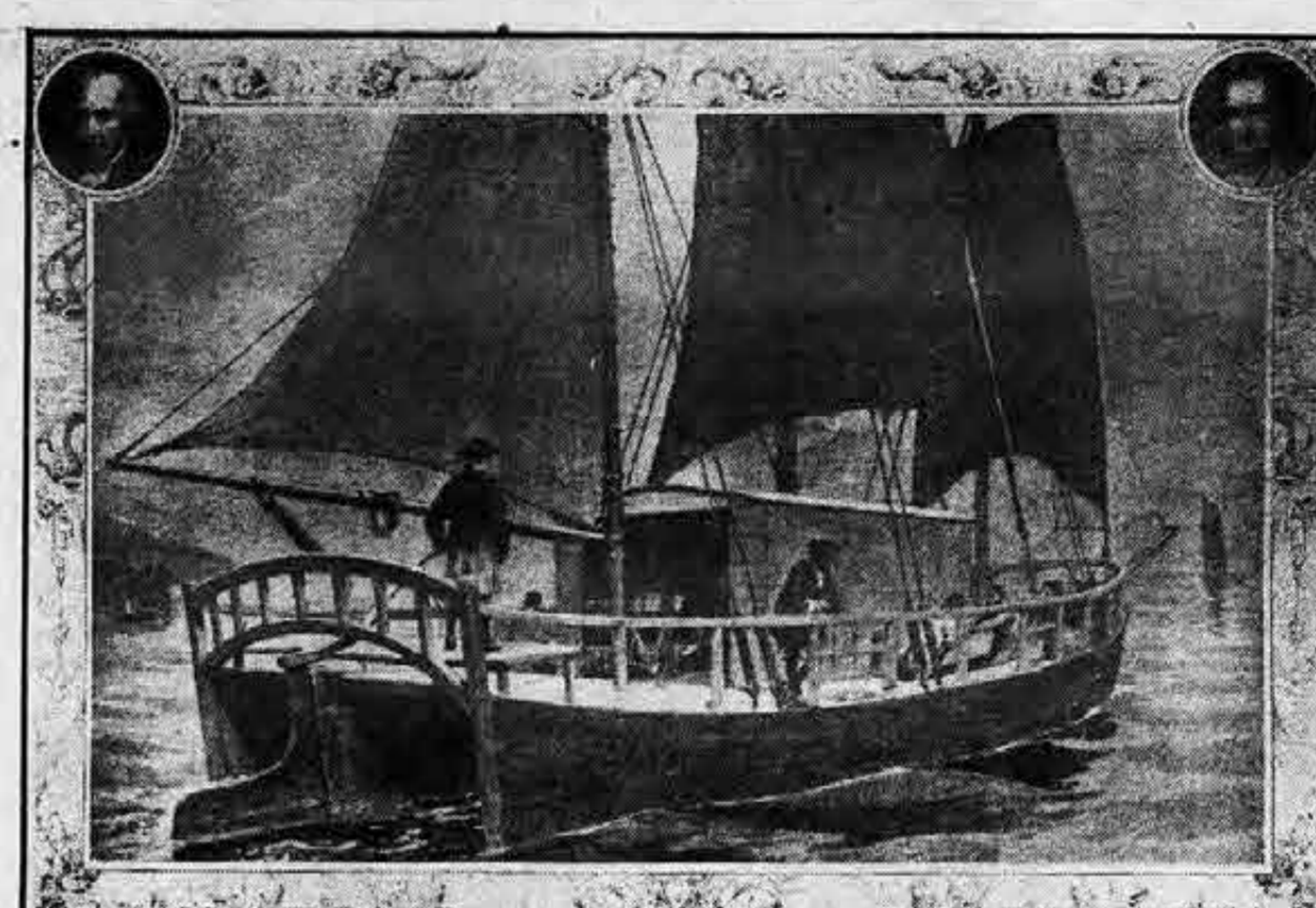
Patrick Miller's double-hulled paddle-boat, built in Scotland (1787). Five paddle-wheels driven by capstans, in tandem between hulls, could be raised out of the water when sails alone were used. The speed was 4.3 knots with 30 men at the capstans.
