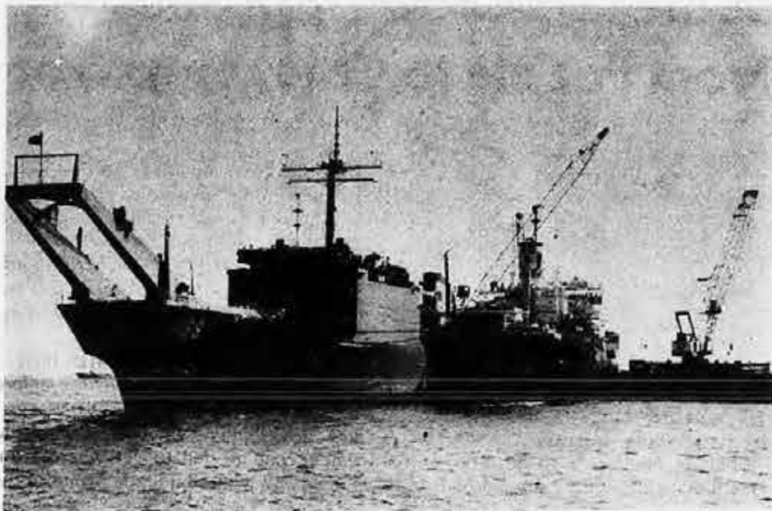
Anchored Sea-Land Warrior (center) shifts containers via cranes to the LST (Landing Ship Tank) (left) and barge (right) in offshore unloading exercise.
