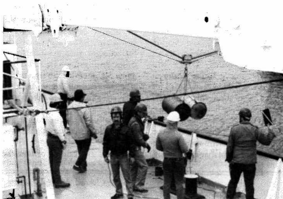
The cargo is picked up and transferred by a highline, to the tank barge.
