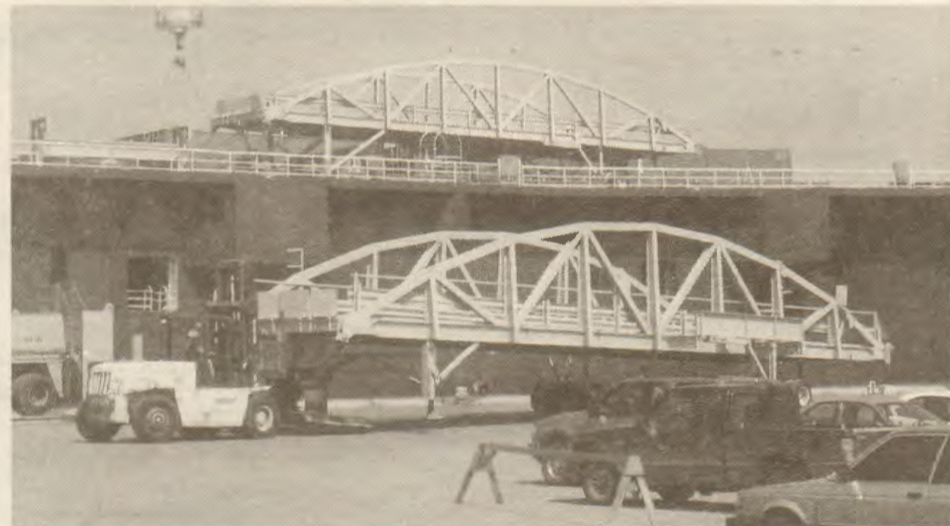
Racks are removed from the El Yunque's deck to be used for RO/RO operations.
