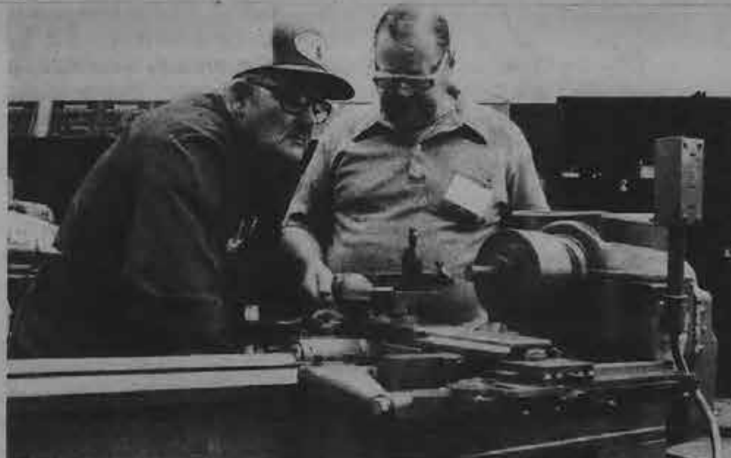
Upgraders Willis Lawrence (l.) and James Henri first adjust the cross slide of the lathe to insure smooth edges and surfaces.
