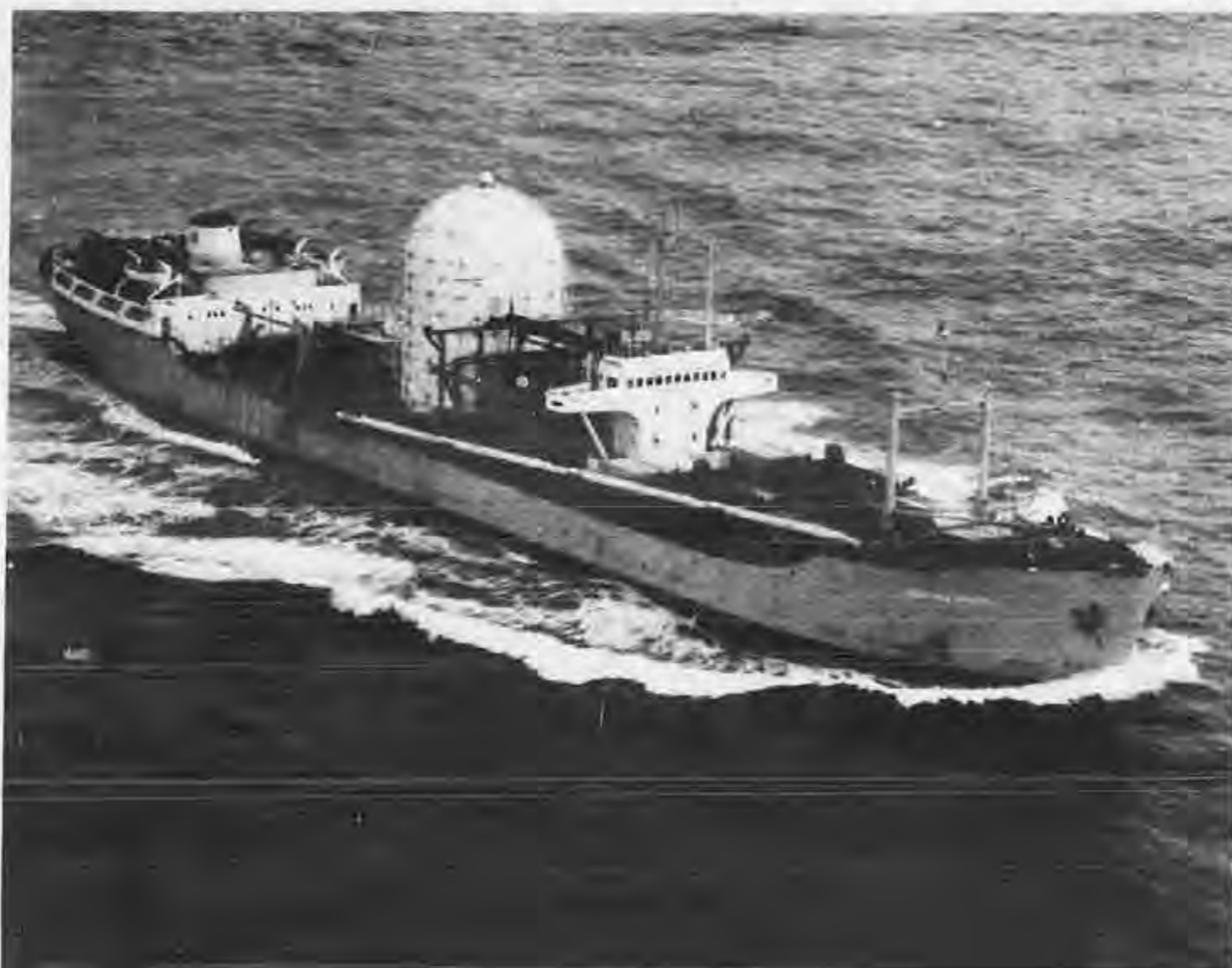
The Deep Sea Miner II, a converted drill ship, now mining the ocean floor, is about one-fifth the projected size of mining vessels that will be used when this new industry gets into full swing.
