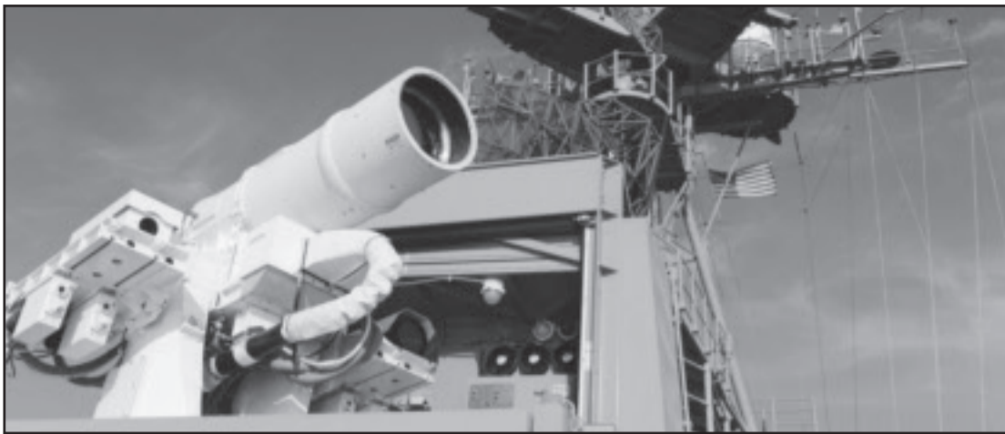
The USS Ponce (photo at right) is shown on deployment in the Arabian Gulf last September. The laser weapon system (LaWS) is visible near the top of the ship, above the bridge. A closer view of the weapon is shown above, in a photo from November. (Both photos courtesy U.S. Navy)
