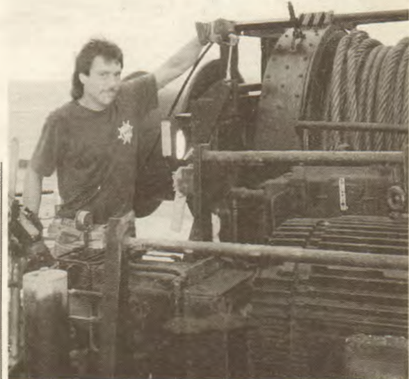
QMED Paul Pagano performs some preventive maintenance—greasing winches—aboard the LNG Leo .
