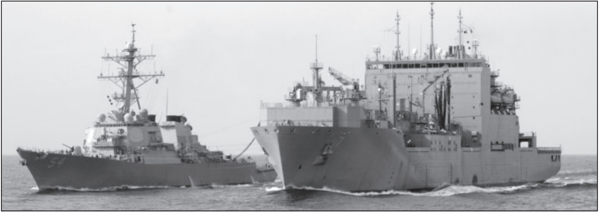
The USNS Carl Brashear (vessel at right above) pulls alongside the USS Curtis Wilbur during a replenishment at sea as part of Operation Tomodachi. (U.S. Navy photo by Mass Communication Specialist 2nd Class William Pittman)
