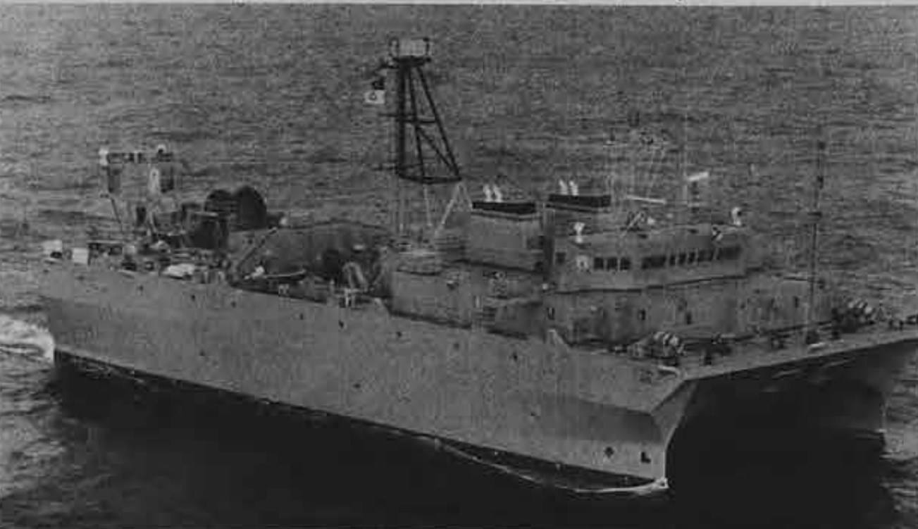
The Able is the second of four new SWATH vessels which can comfortably operate in high sea states.
