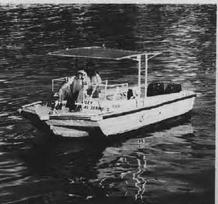
One of the many Crowley skimmers operated by Seafarers heads into the oil-fouled Atlantic Ocean. The boats were used to position booms and gather oil.
