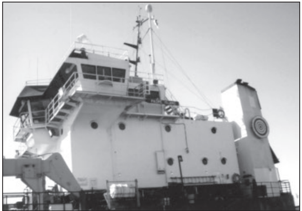
Operated by Great Lakes Dredge & Dock, the Padre Island is a trailing suction hopper dredge and is 281 feet long.
