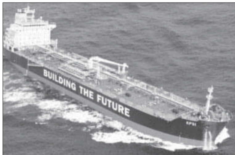
This artist's conception of the Kvaerner Philadelphia tankers reflects the vessels' 600-foot length and 46,000 deadweight tonnage.
