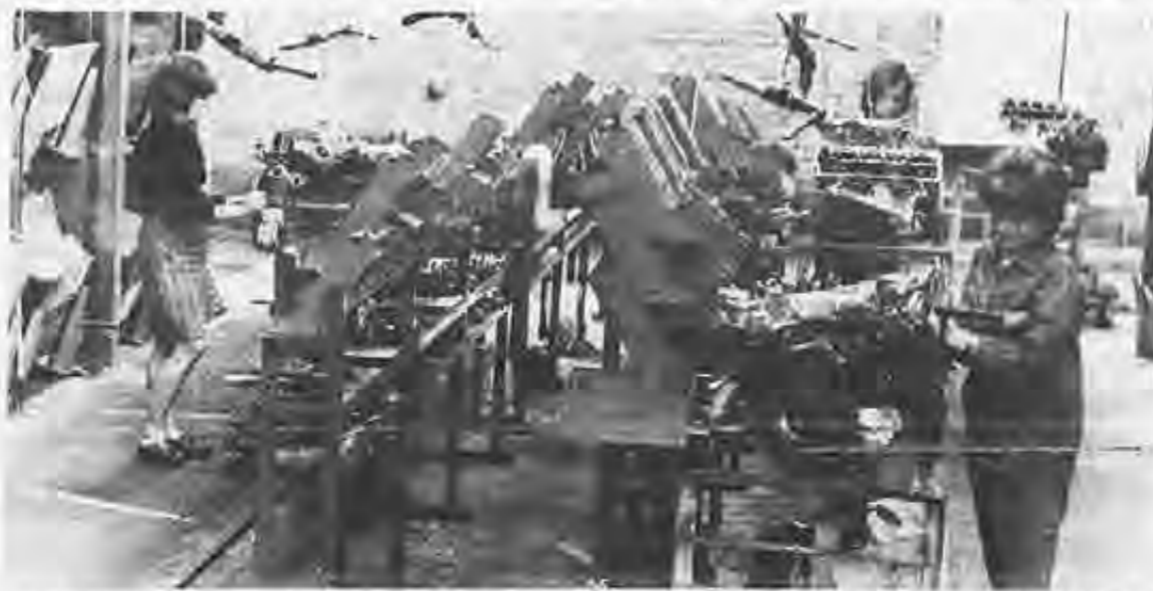
The above photo shows part of a new work form at Saab-Scania called group assembly. Instead of being on the traditional assembly line, these workers are members of a group helping to assemble a truck diesel engine. They decide among themselves how the work is to be distributed.
