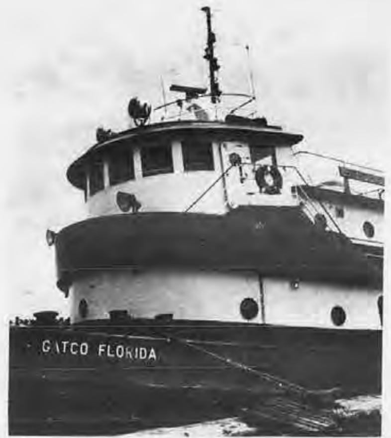
The Florida is GATCO's only deep sea tug. The 3,000 hp. boat runs from Mobile to San Juan.
