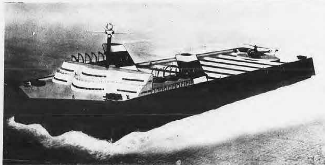
Artist's representation of The Stradler making a voyage with 10 fully-loaded barges which will be swapped for 10 others, also fully loaded at the landing end. Operation will require 30 barges, 10 in transit plus 10 more at each end, for each of the catamaran motherships operated in the rapid service.
