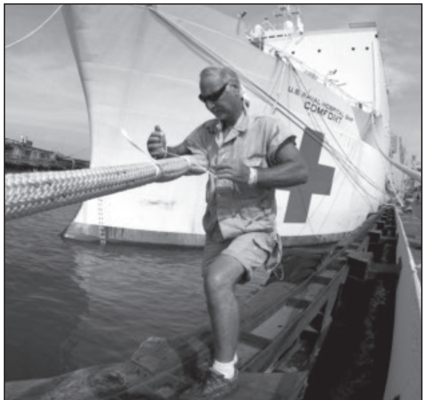
Bosun Gerald Butch places chaffing gear on mooring lines as the USNS Comfort is docked in El Salvador. (U.S. Navy photo by Mass Communication Specialist 2nd Class Eric C. Tretter)
