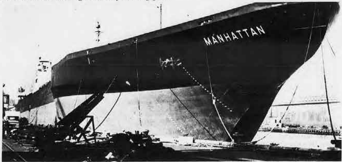
Note the unusual ice bow of the S/T Manhattan when she was moored at the old Navy Yard, now the Seatrain Shipyard in Brooklyn, N.Y.
