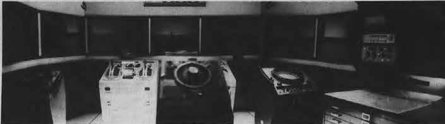
Pictured here is a full view of the SHLSS ship simulator bridge, as the students see it, with radar scopes, helm controls, radio and navigation aids. Not pictured is a rear projection screen which allows students to see what's happening aft.
