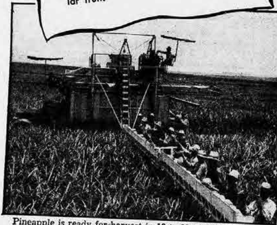
Pineapple is ready for harvest in 18 to 22 months. Pickers drop ripe pineapples on 50-foot conveyor belt which transfers the fruit into the truck bin.
