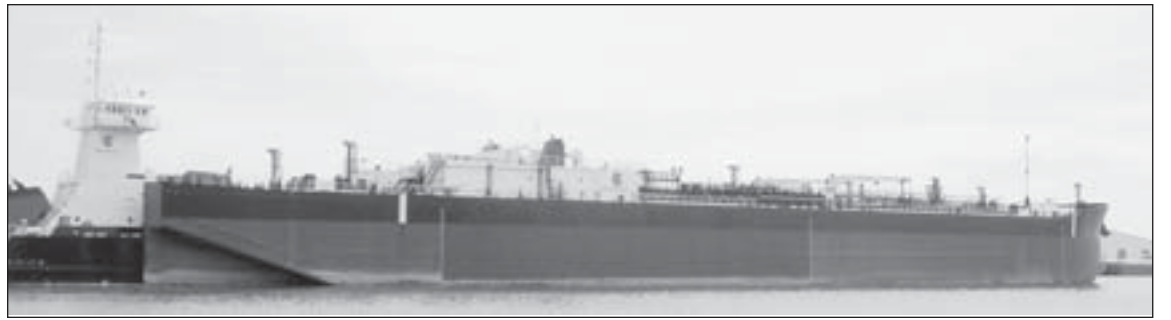
The new ATB features all the latest equipment and double-hull construction.
