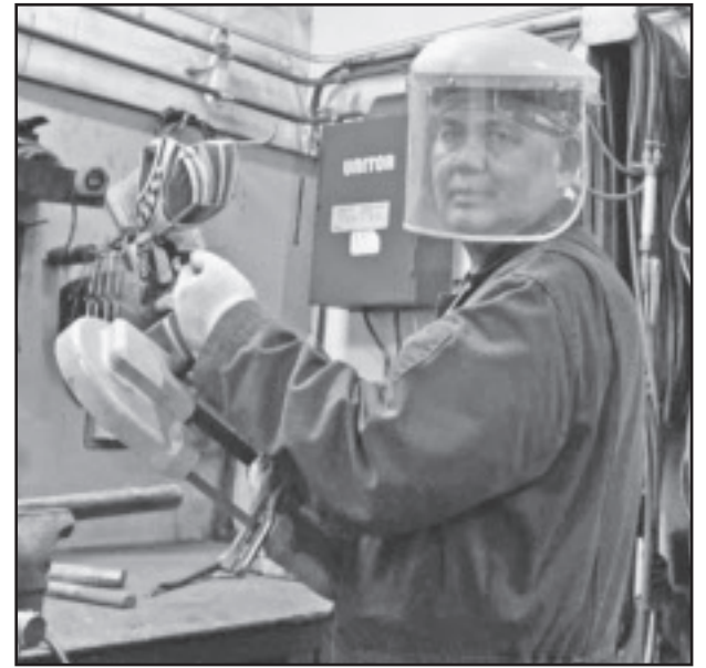
ABOARD MAERSK DURBAN – QMED Sammy Montana cuts a metal pipe fitting with an electric jigsaw.
