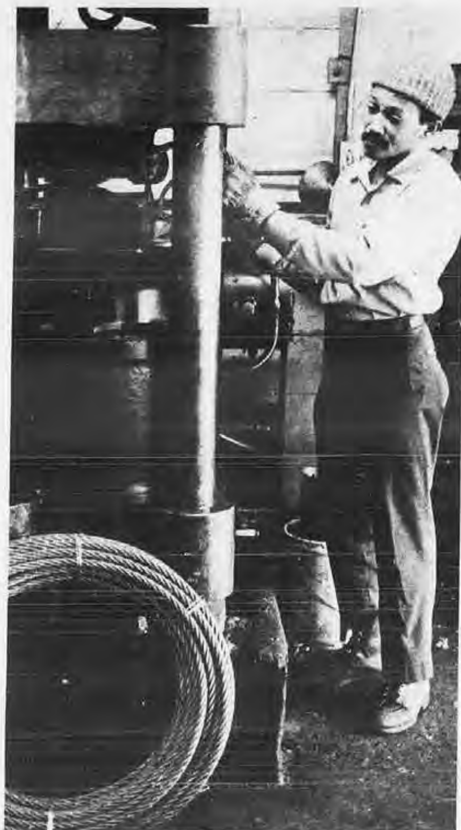
Paulsen Wire Rope also has a hand in New Orleans port activity. Shiploading lifts and slings are fashioned in this shop, which has been organized by the United Industrial Workers, an affiliate union of the SIU. UIW splicer Raymond Penns is shown here putting a cargo runner through the hydraulic press.
