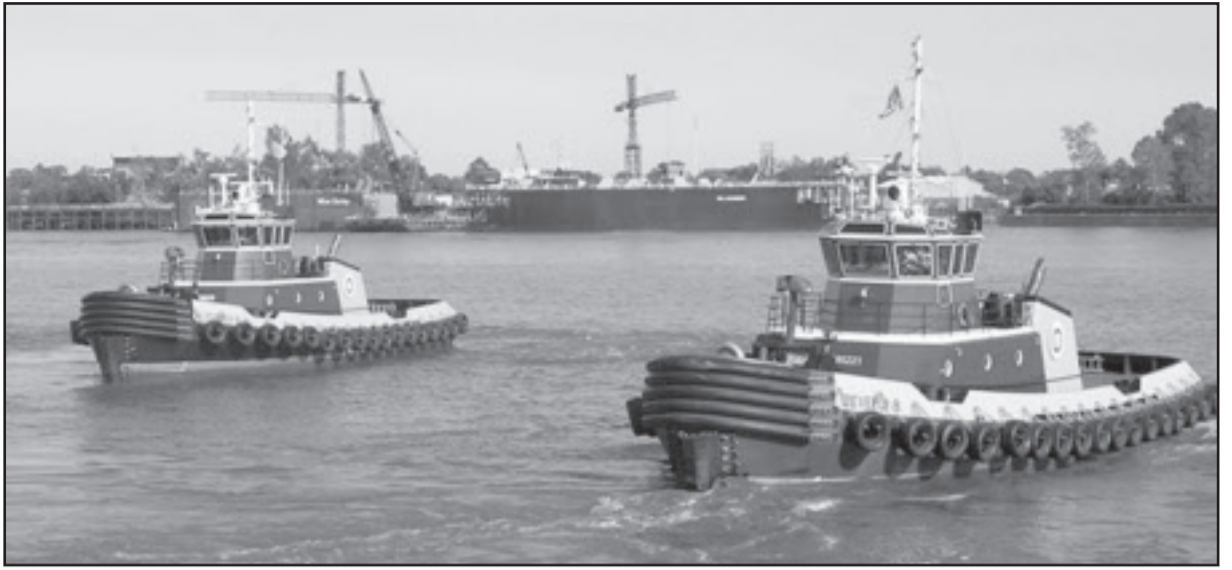
NEW TUGS FOR BISSO FLEET – Seafarers-contracted E.N. Bisso & Son Inc. in December welcomed two new Z-drive tugboats into its fleet in New Orleans: the Elizabeth B (left) and Beverly B . Each boat measures 96 feet in length and 34 feet in beam. According to a news release from Jensen Maritime, which designed the boats, the tugs “are powered by twin Caterpillar 3516-C Series II main engines that produce a total of 4,000 BHP....” Approximately 60 SIU members sail aboard Bisso tugs.
