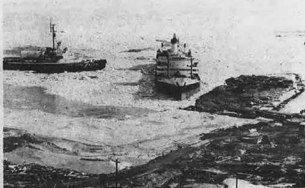
The tanker USNS Maumee becomes the longest and largest ship to tie up at the man-made iceberg wharf in McMurdo Bay, Antarctica—the bottom of the globe. At left, the 269-foot USCG icebreaker Staten Island stands by after clearing a path through the ice for the docking ship.
