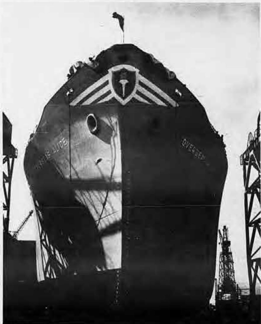
The latest addition to the roster of SIU-contracted ships is the Overseas Alice, owned by Maritime Overseas and constructed at the Bethlehem-Sparrows Point Shipyard in Baltimore. She has a deadweight of 37,050 tons, is 660 feet long, and puts out 15,000 horsepower.
