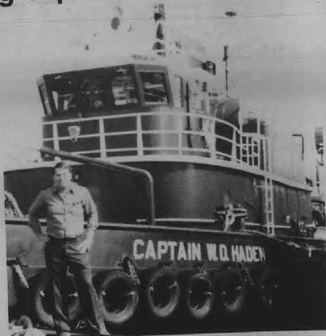
Bay Houston Towing Co. VP Norman L. Conner proudly poses in front of the 106-foot, 13-knot Capt. W.D. Haden . She can comfortably berth 10 crewmembers in five staterooms.
