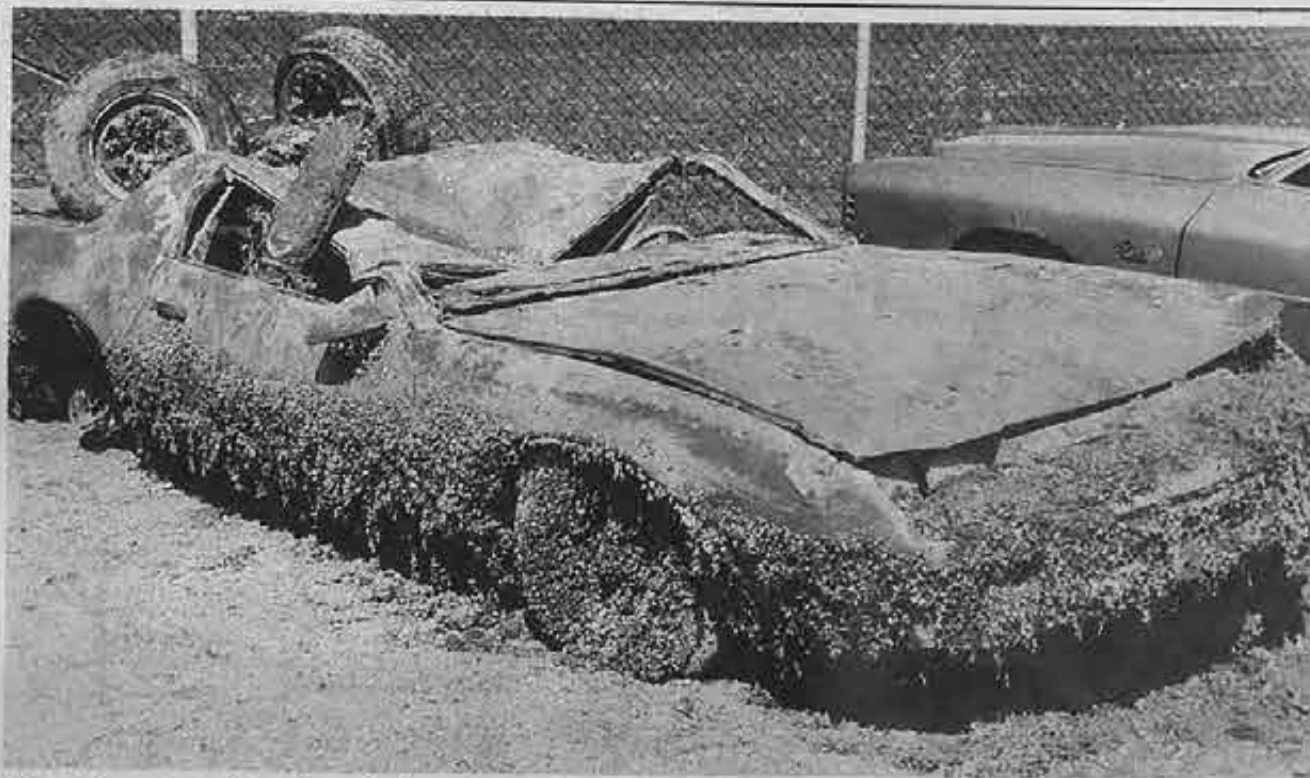
The zebra mussel is not particular about what surface it attaches to. The adaptable organism sticks to ships, tugboats and more. Shown above is the effect of the striped mollusk on a car which was submerged upside down in Lake Erie for a year.
