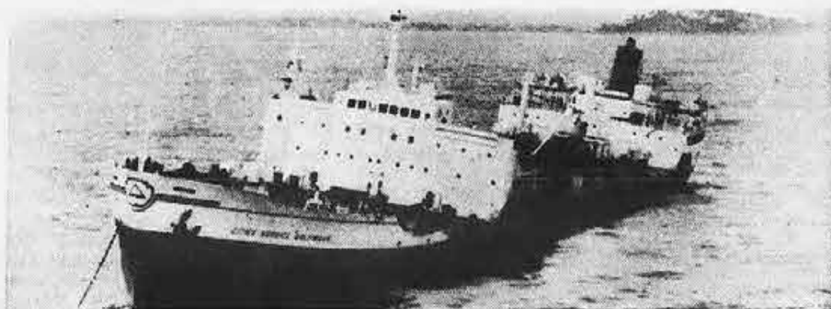
The SIU-manned tanker Cities Service Baltimore lists 20 degrees to port after a 300 to 400-foot gash was ripped in her side below the waterline when the vessel struck an underwater ledge in Boston Harbor recently. (Story On Page 2.)
