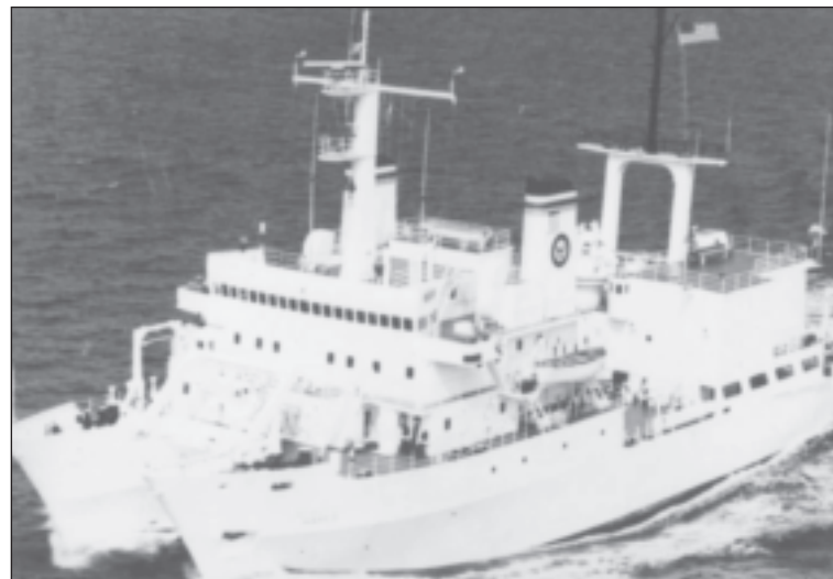
The USNS Hayes is equipped with two auxiliary propulsion diesel engines for use during acoustic operations.
