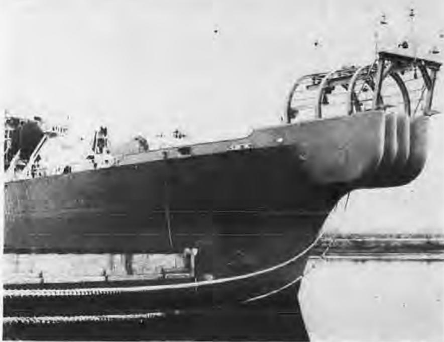
Above is a front view of *Long Lines* tied up at its home base in the port of San Diego, Calif. Note the caged, protruding bow of the cable-layer and two deck marker buoys on the starboard side.
