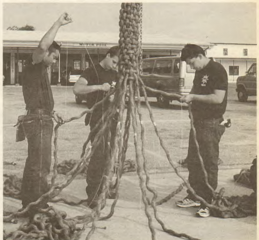
Lundeberg School students from class 539 of the entry level training program practice the intricate rope work involved in making a fender for one of the school's training vessels, Little Toot . From the left are Orlando Sierra, Justin Vieira and Josh Cannizzaro.
