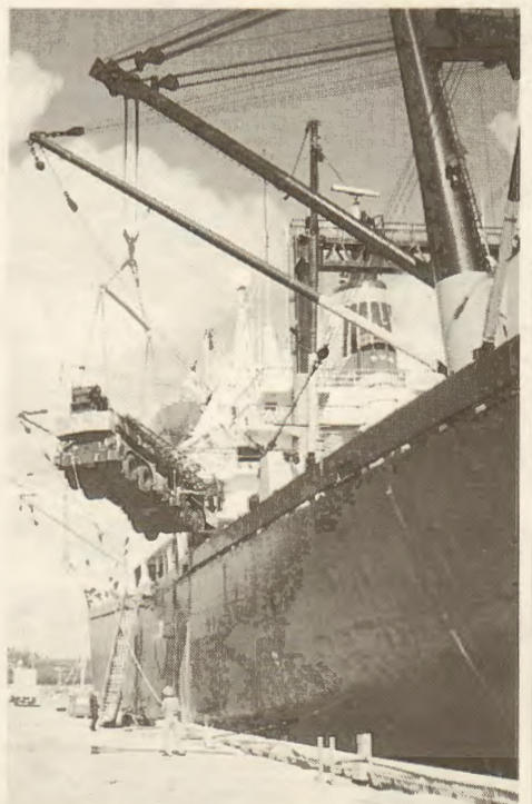
The Cleveland's jumbo boom—capable of lifting 70 tons—unloads a military vehicle in the port of Guam.
