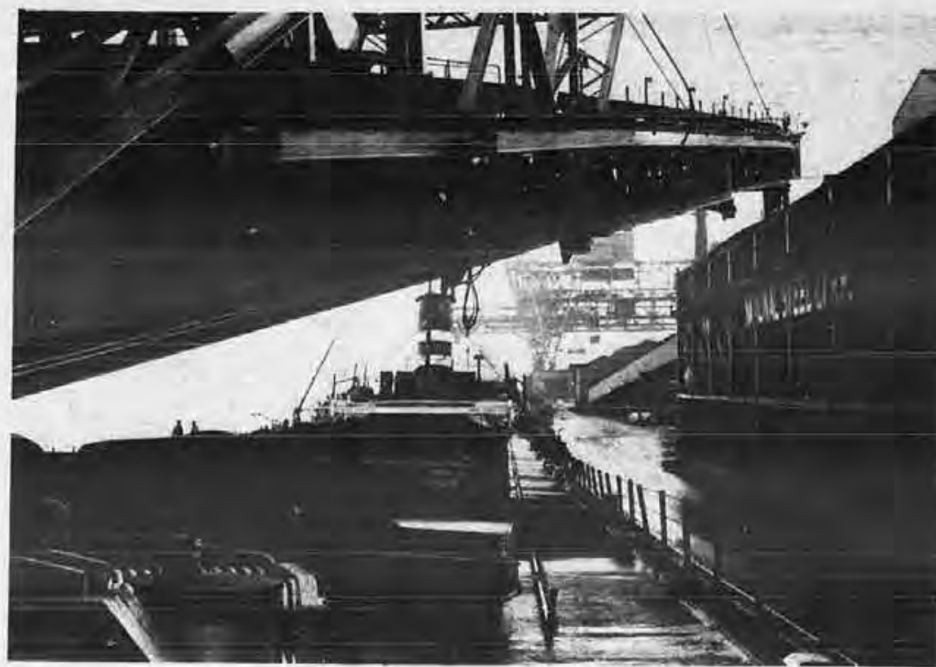
The M/V Richard J. Reiss ' conveyors unload the coal the ship brought into Detroit.
