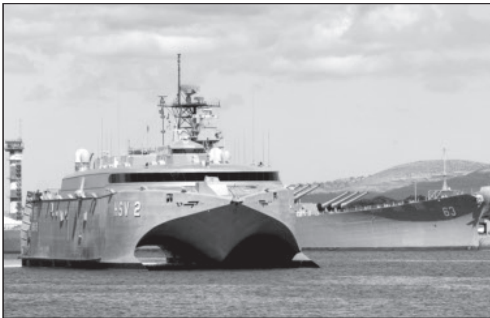
The Seafarers-contracted Swift , pictured near the battleship USS Missouri in Pearl Harbor, Hawaii, is a versatile vessel that can sail at up to 42 knots.
