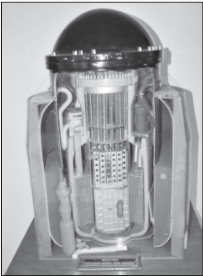
Cutaway model of the Savannah's nuclear reactor
