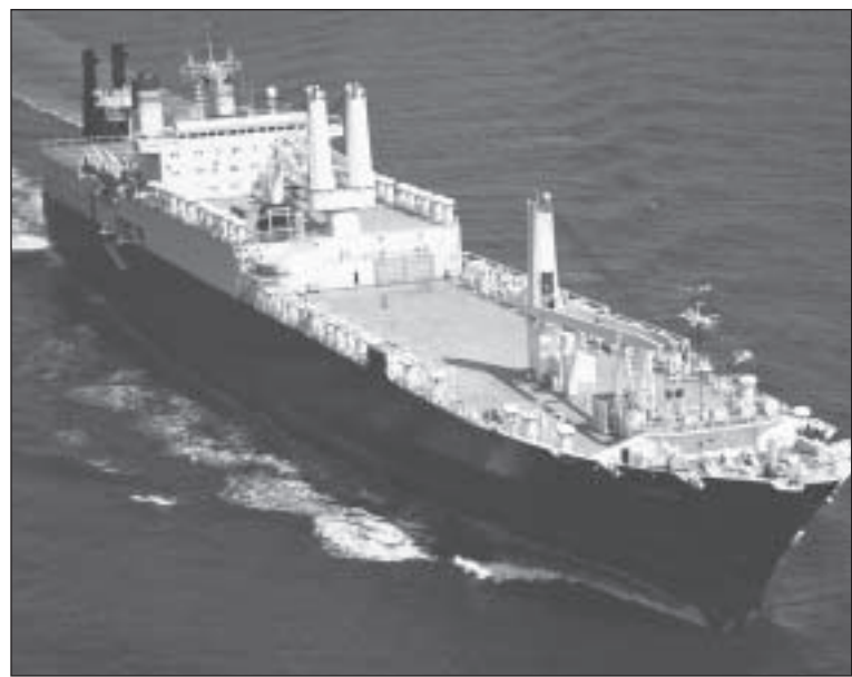
The prepositioning ship USNS Wheat has a total cargo capacity of 200,000 square feet and can sustain speeds of more than 20 knots.
