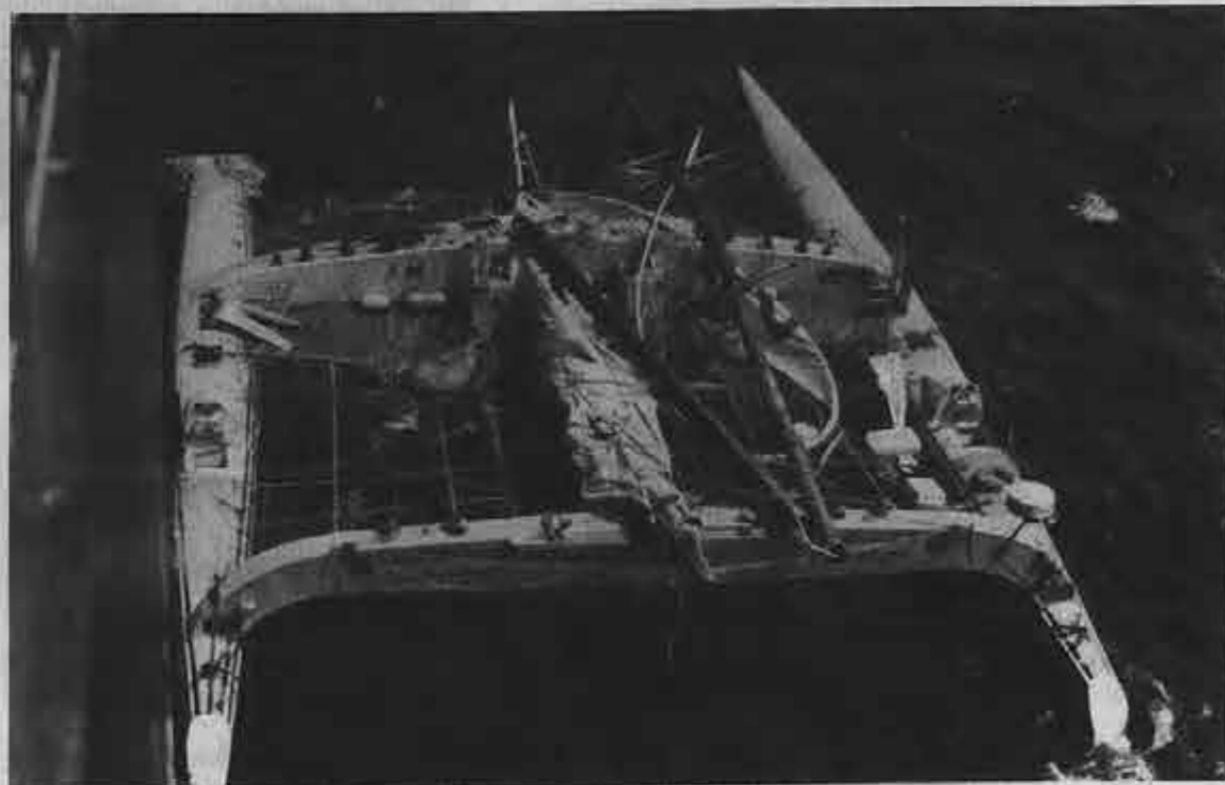
The Chaffoteaux Challenger is pictured above as it was seen off the side of the Sea-Land Performance following its rescue after a storm had snapped its 100-foot mast. Right is a view of the catamaran under full sail.
