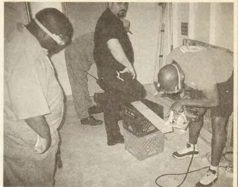
Above: During damage control training aboard the American Queen , crewmembers construct wooden patches to cover ruptures in the boat's hull. From the left are Deckhand Bryan Johnson, Deckhand Kenya Lewis, Engineer Randy Dominique and Deckhand Mike Ward.
