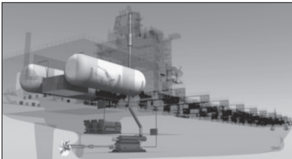
An artist's rendering highlights the propulsion system of TOTE's new LNG-powered containerships. (Photo courtesy NASSCO)
