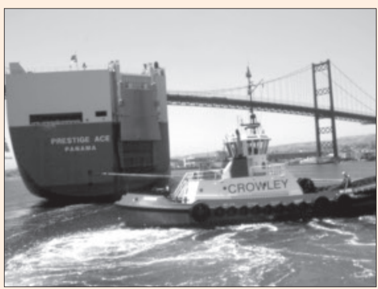
The harbor tug Master maneuvers in "indirect mode" (traveling sideways) to slow an outgoing car carrier in Los Angeles/Long Beach.
