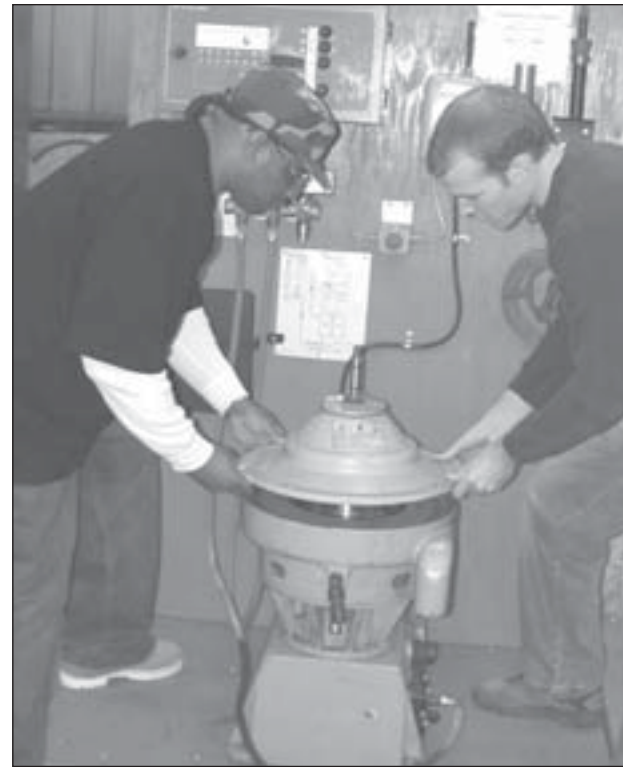
Therman Ames III (left) and Kenneth Ross (right) practice lube purifier maintenance.
