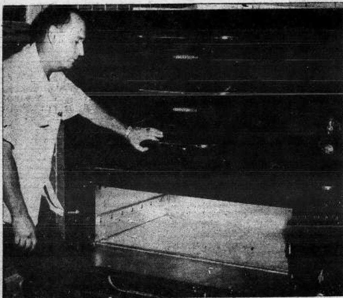
Frenchy Michelet, who has been overseeing the work on the building, inspects a Blodgett oven, which is one of a number of units in the SIU galley and bakery, with an aggregate capacity of 100 large Pullman loaves of bread at a single baking.
