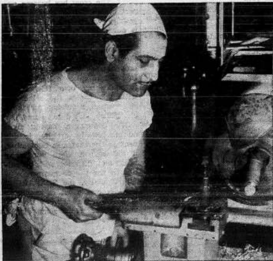
Paolo Pringi, Oiler on the Beauregard, wheels the cutting tool into place as he prepares to turn down a brass rod on the ship's lathe. The excellent photo was by a shipmate using a speed graphic.
