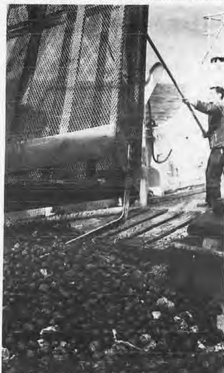
Research vessels use a simple dredge bucket and line to bring up samples of the nodules. (courtesy Kennecott Copper)
