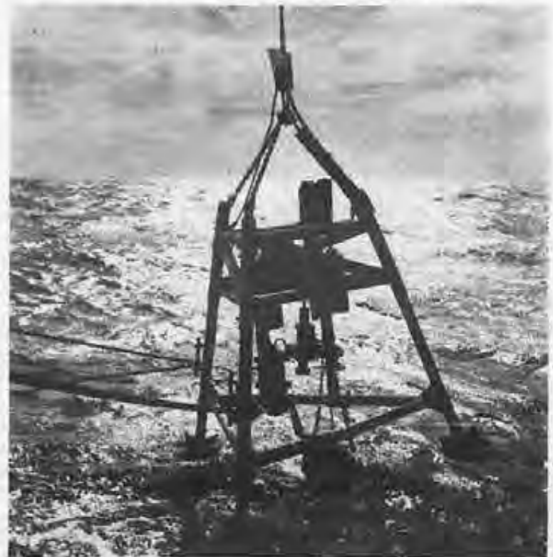
Camera and lighting equipment attached to tripod are lowered into the ocean in the search for nodule concentrations. (courtesy Kennecott Copper)
