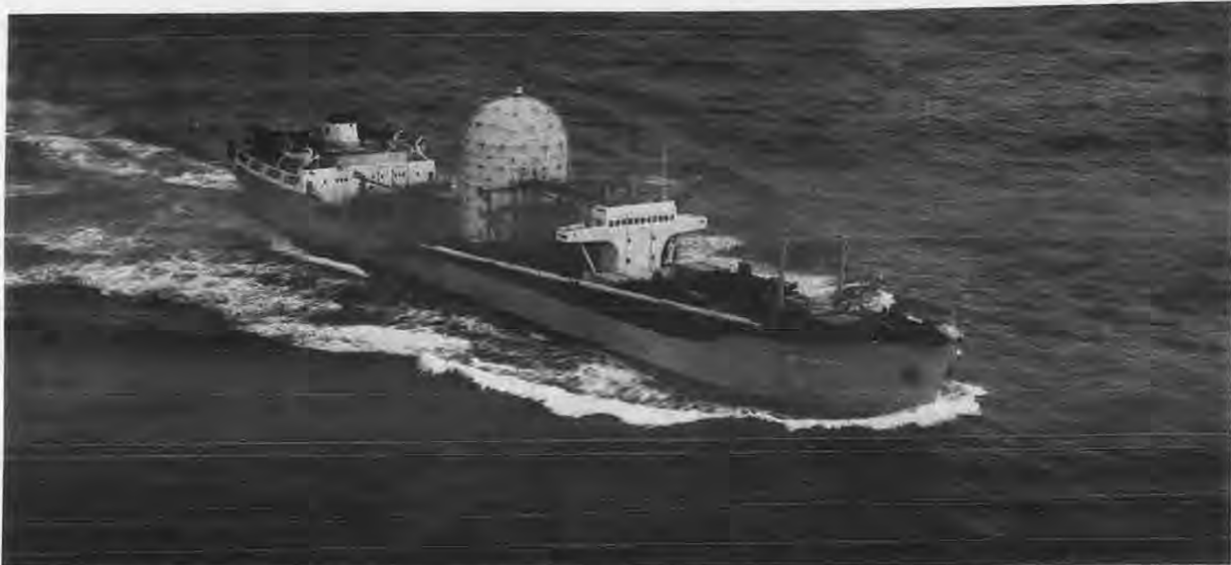
The Deep Sea Miner II, a converted drill ship, now mining the ocean floor, is about one-fifth the projected size of mining vessels that will be used when this new industry gets into full swing. (courtesy Deepsea Ventures)
