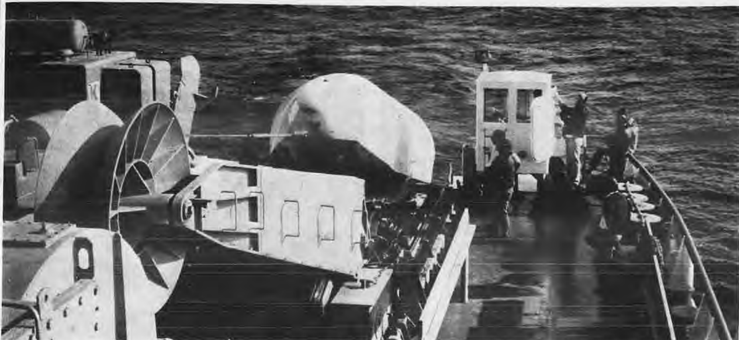
Researchers lower one of several types of nodule collectors off stern of mining vessel. This particular collector is designed to gather the most nodules while raising the least amount of sediment and using the least amount of power. (courtesy Kennecott Copper)
